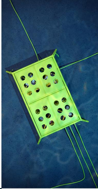
The repeated expansion and contraction of pipe lines fixed to the subsea PLET's often causes the base to dig into soft silt, resulting in unacceptable stress levels building up in the attached pipe lines over a period of time.
